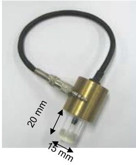
Suction probe (total of 18) Soil Water Potential: +700 to -90 kPa, \pm 0.5 kPa
