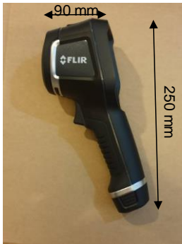
Thermal camera (total of 1) Resolution 120 \times 90 pixels Object Temperature: -20° to 250° C, \pm 2 ° C
